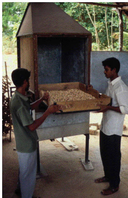
Figure 6: The Practical Action Tray Dryer in Sri Lanka ©Practical Action/Zul
