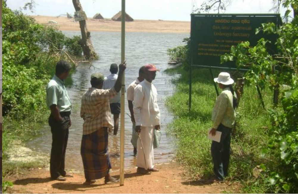
Installation of flood gauges
