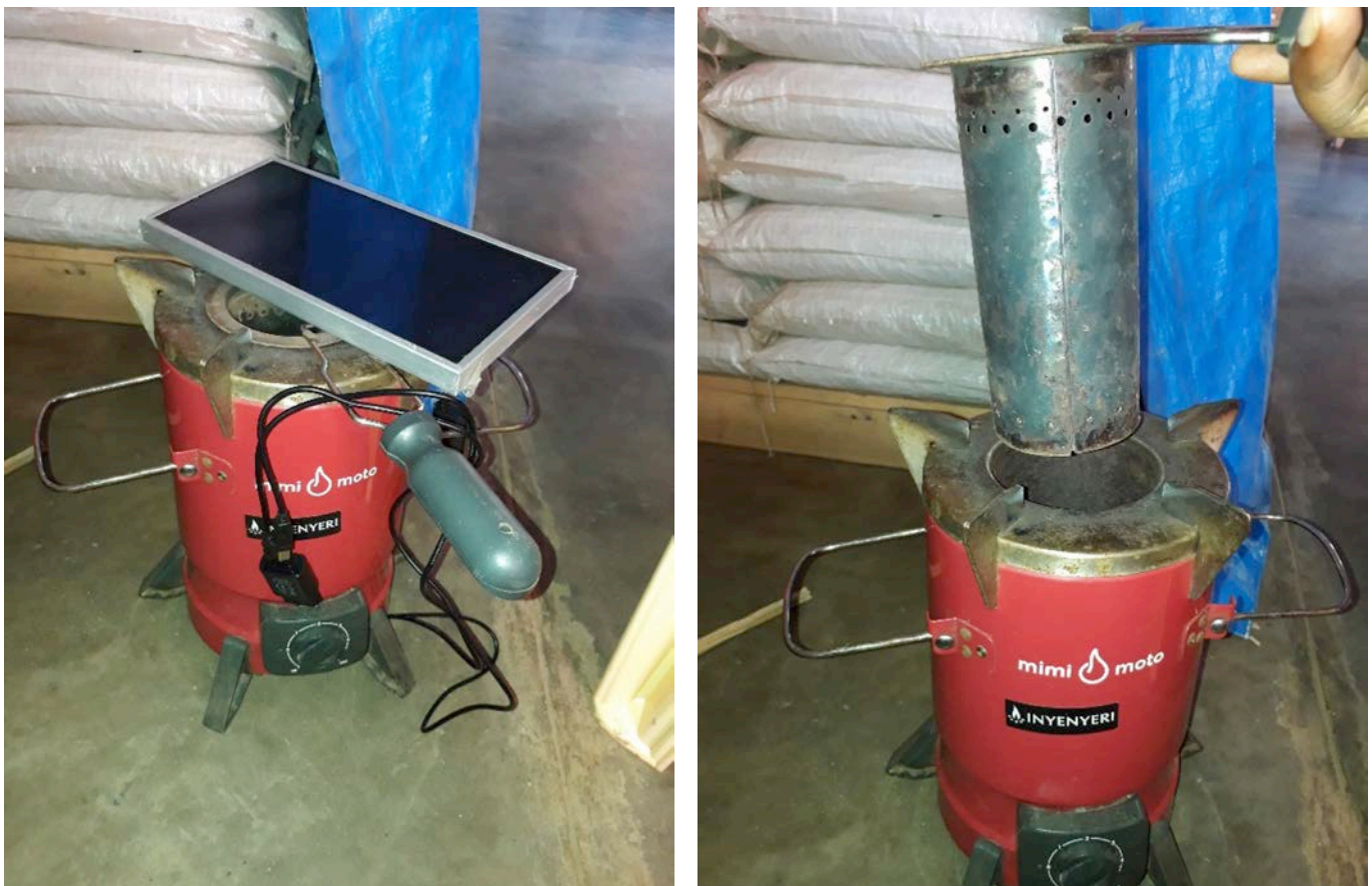
Figure 5.4 The Mimi Moto pellet stove distributed by Inyenyeri in Kigeme, showing (left) the solar panel used to power the fan and (right) the burning chamber of the stove
