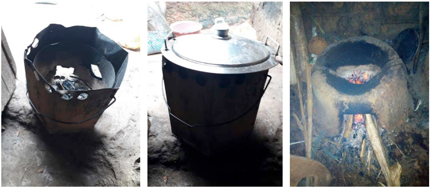
Figure 5.3 Save80 cookstoves distributed by UNHCR in Kigeme Camp (left, centre) and a Rondereza stove (right)
