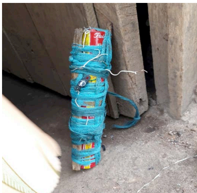
Figure 4.2 Improvised torches made from salvaged non-rechargeable batteries (left) and affixed to a roof beam to provide space lighting (right)
