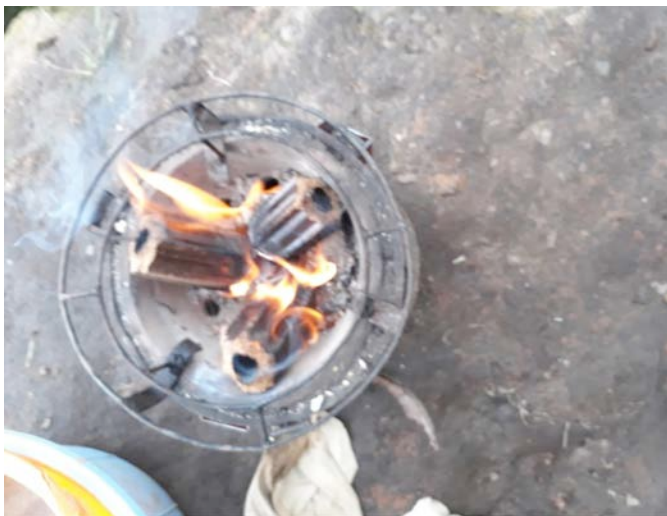
Figure 5.6 Briquettes from Bamboo Riverside in Kigeme that produce a flame like firewood at first (left) and then smoulder like charcoal (right)
