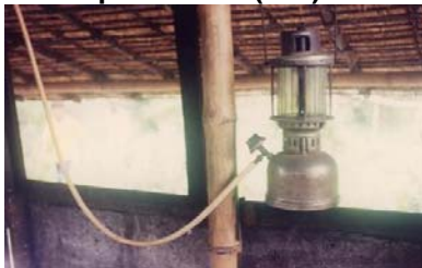
Hajjak light based on biogas
