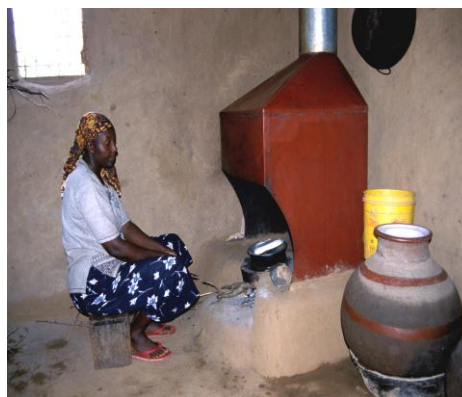
Figure 3: Woman cooking with her stove and smoke hood, Kenya. Photo credit: Practical Action East Africa
