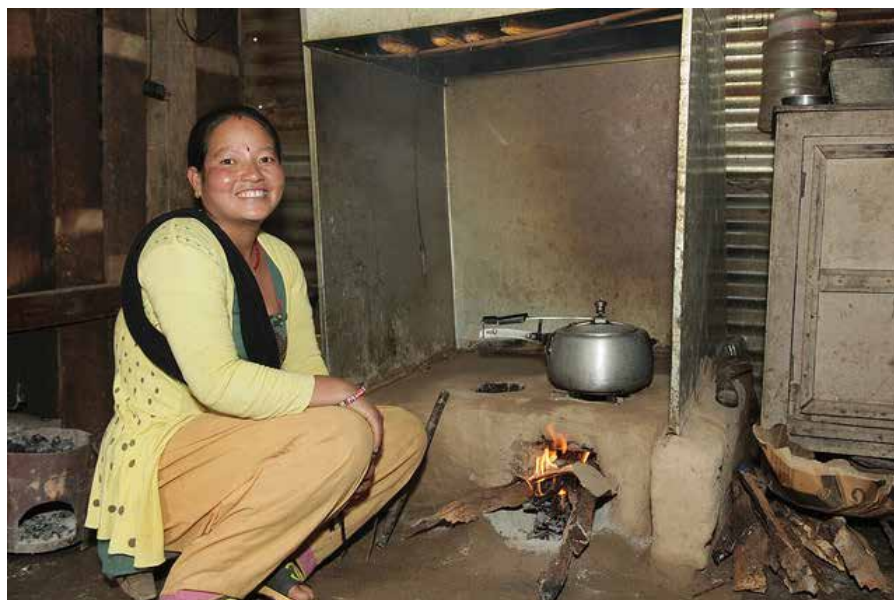
Saraswoti Bal, a villager from Dhading District using an improved cookstove and smokehood which can reduce exposure to household air pollution by as much as 82%
